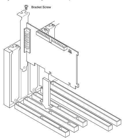
Figure 1.2 Inserting the Host Adapter
